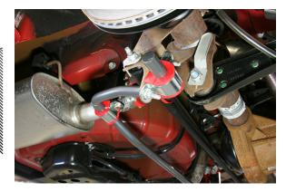
21. Before tightening the remaining hardware, ensure the sway bar is centered from side to side between all four bushings. Torque all four bushing bracket bolts to 52 ft lbs. Torque the upper end link bracket bolts to 85 ft lbs.
