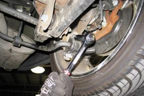
9. Remove the 18mm bolts from the upper end links. Leave the mounting nuts, which are secured by clips, attached to the chassis.
