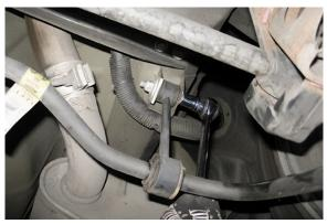
10. Detach the original equipment sway bar assembly from the vehicle.
